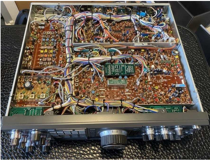
Under the cover of a Kenwood TS-940S, lots of analog circuits, (transistors, coils, capacitors, filters, etc.)
